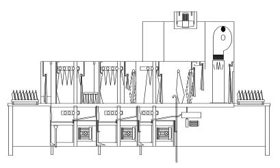
Figure 1: A typical multi-tank dishwasher (dishes enter the machine at the left)
